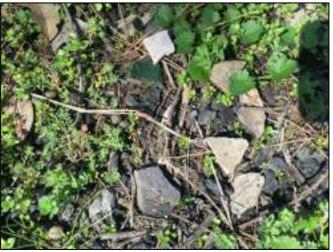
Plate 22 – Fragments of burnt fibre cement sheeting in area of burning.
