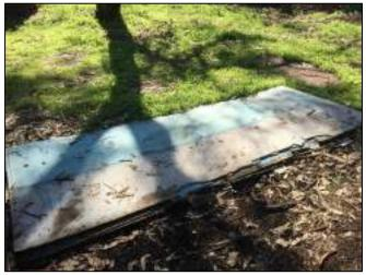
Plate 10 - Sheets of fibre cement sheeting. Did not appear to be ACM.
